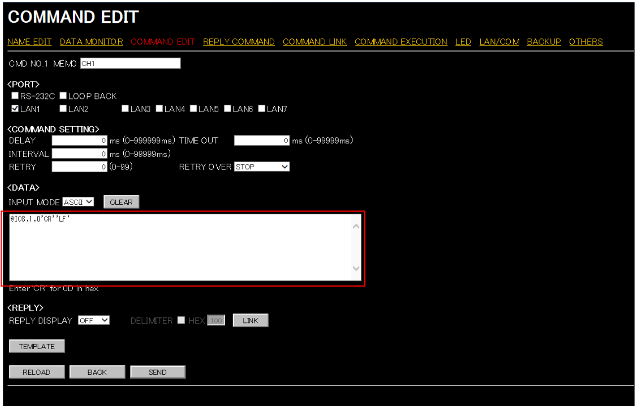
[Fig. 9.17] Control command has been input using input support
