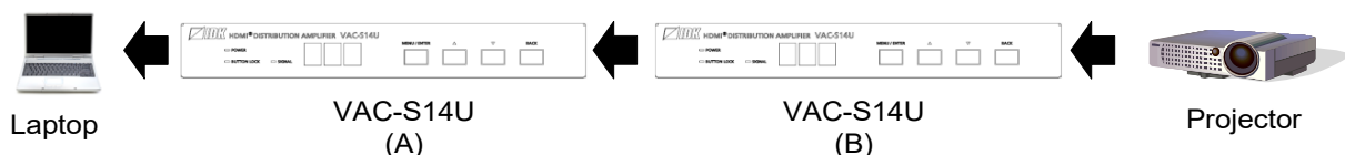
[Fig. 8.4] Reading EDID in cascade connection
